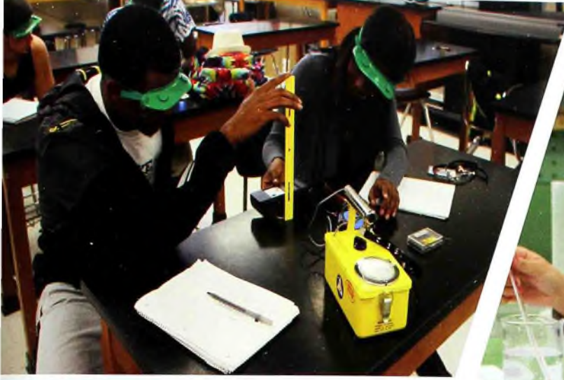
Scientific Relationships Senior Angelo Donovan and junior Tabitha Holmes work together on an experiment in their Nuclear Science class. This experiment represented the relationship between radiation and distance using a radioactive source and a Geiger Counter. Each distance from the table was recorded and analyzed. They were able to explain why different shielding was useful to block radiation. Photo by Lucia Juarez
